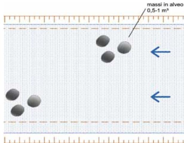
FIG. 6-23 MASSI DISPOSTI A TRIANGOLO.
